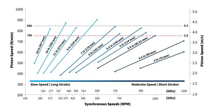
Ariel's moderate-speed process compressors operate in comparable piston speed ranges to long-stroke,
